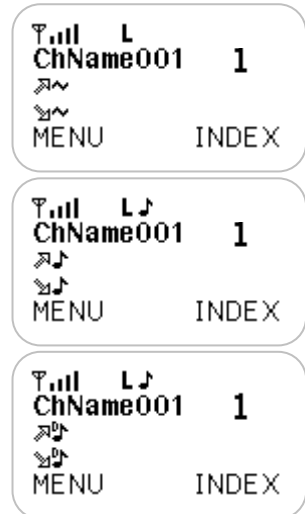
Figure 4.8 – Analog receive display
