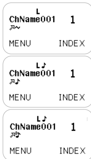
Figure 4.13 – Analog transmit displays
