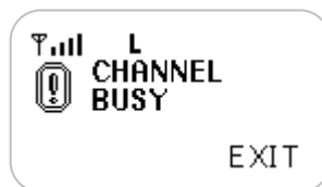
Figure 4.17 – Busy channel lockout
