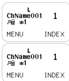
Figure 4.15 – Encrypted transmit display
